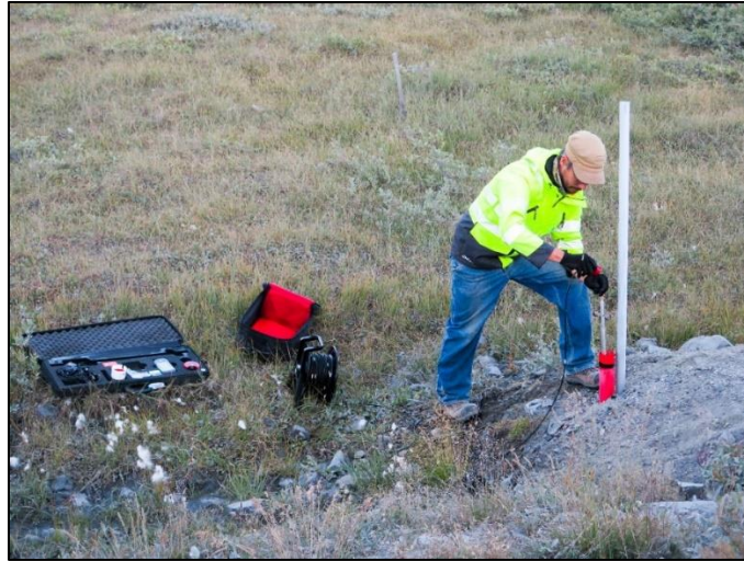
Figure 18 : Taking measurements at a vertical inclinometer located at the road embankment toe.
