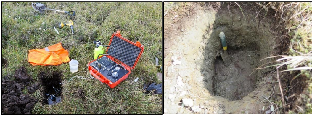
Figure 16 : (Top): Measurements of the critical shear stress of permafrost with a Cohesive Strength Meter (Bottom): Levelling of the permafrost surface prior to make a test.
