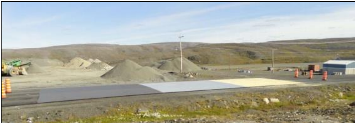
Figure 19 : High albedo coatings after their implementation on September 1 st , 2015 (Richard, 2018).
