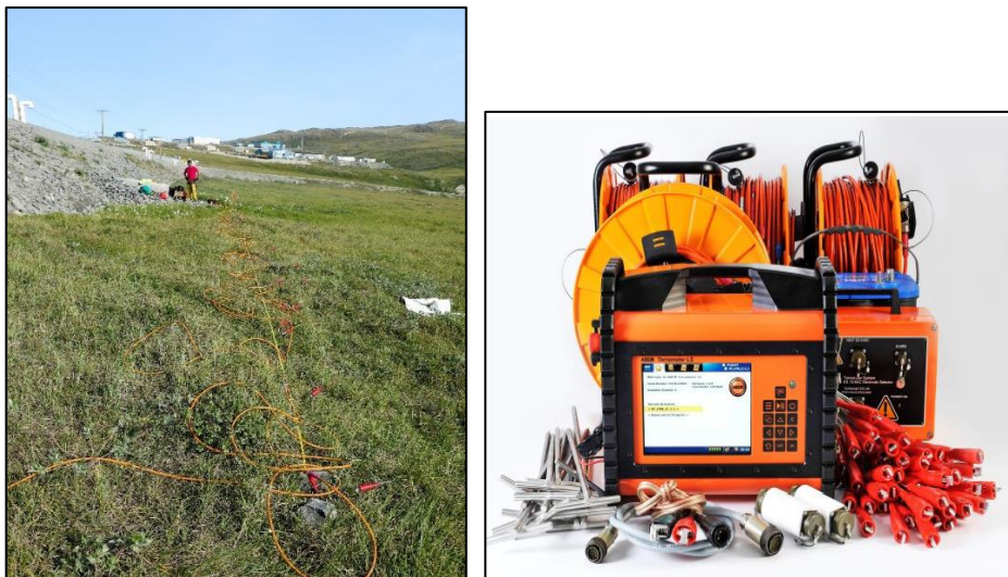
Figure 10 : (Left) ERT survey at a culvert outlet; (Right) ABEM Terrameter LS.
