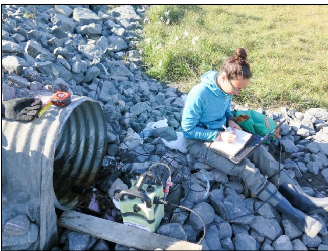
Figure 9 : Water flow measurements at the outlet of a culvert.
