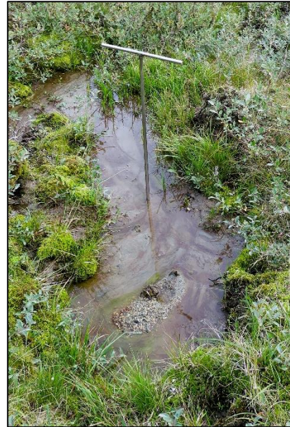
Figure 7 : Thaw depth measurements with a frost probe.
