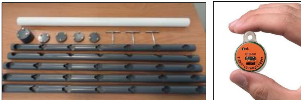
Figure 21 : PVC tubes and temperatures sensors #UTBI-001 used for this research project (Richard, 2018).
