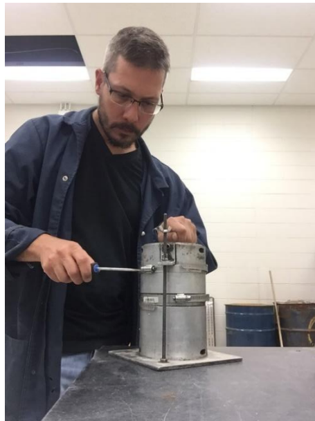
Figure 22: Molding of a Saluit soil sample in preparation of a frost heave test.
