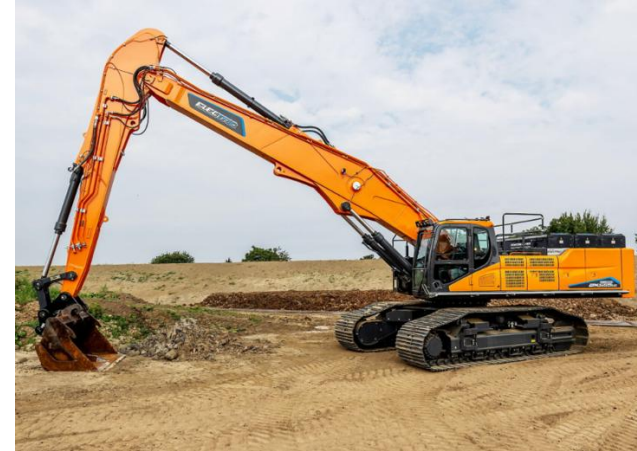
Develon 55 ton battery electric excavator, converted by Staad, NL, 2025,
