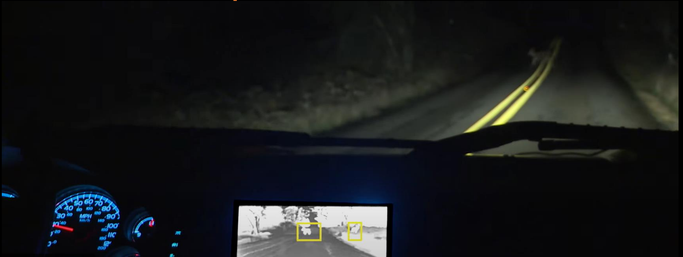
Figure 9 - Vehicle infrared technology can detect deer and other heat-emitting objects and transmit the information to the driver's display. Source: Teledyne Flir
