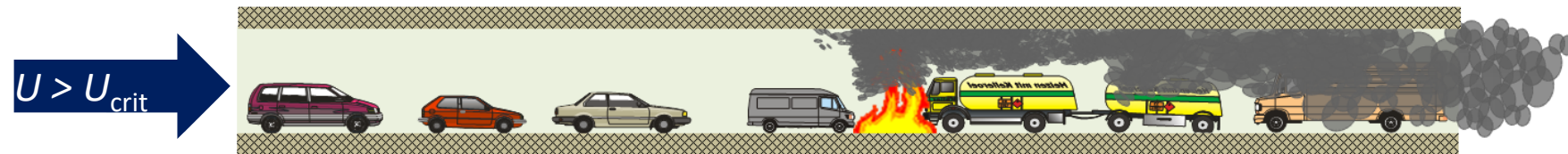
B: Longitudinal ventilation, no smoke backlayering: smoke spread only in one direction, smoke dilution
