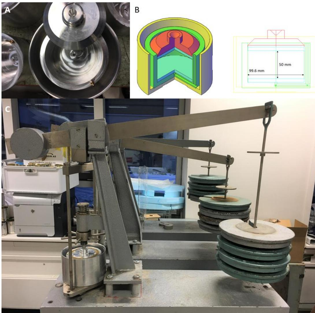
Figure 7: Laboratory set up: A) Compaction mold made at NTNU; B) Schematic of the mold with dimensions; C) Oedometers used.
