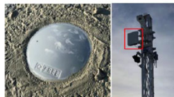
Magnetometer sensor (left) and mast station (right) (image: Q-Free)
