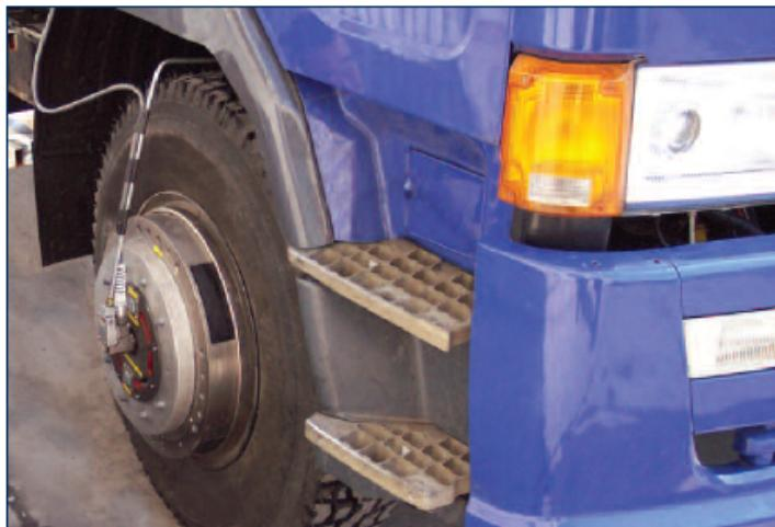
PCB® Series 5400 Wheel Force Transducers are designed as rugged, one-piece sensors that mount between the vehicle hub and the wheel rim, delivering highly accurate road load data measurement and superior performance in a durable water-resistant package. Possessing superior temperature compensation properties and integral overload stops, these sensors provide a high level of confidence in data acquired during aggressive road events, including heavy braking tests.
