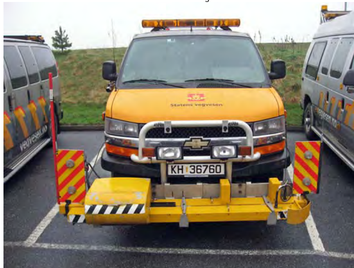
Beam technology with 17 Ultrasonic Sensors!
