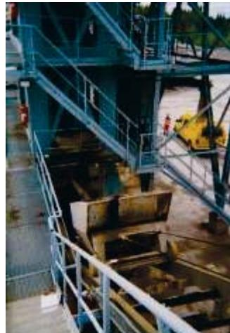
**Figure 2 Mixture-filled dog being pulled up to silos**
