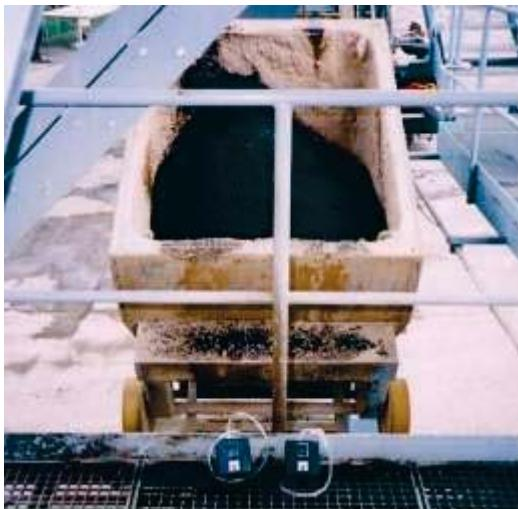
**Figure 5 Samplers on landing**
