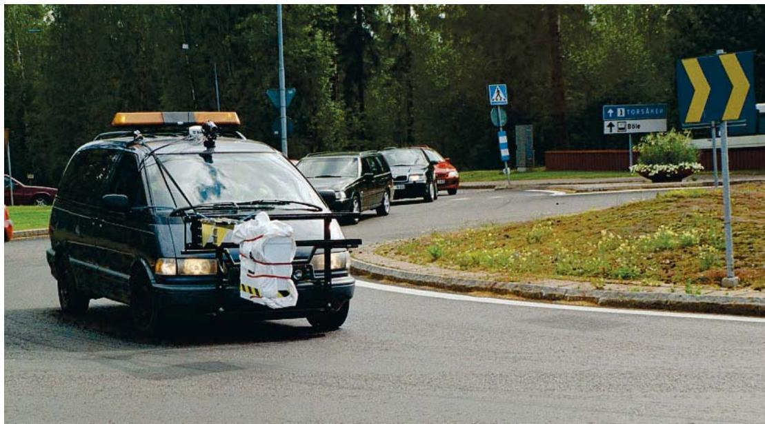
Figure 3. A GPR horn antenna system.
